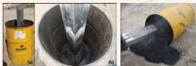
Biochar Kiln: a) external view, b) internal view, c) Produced biochar
